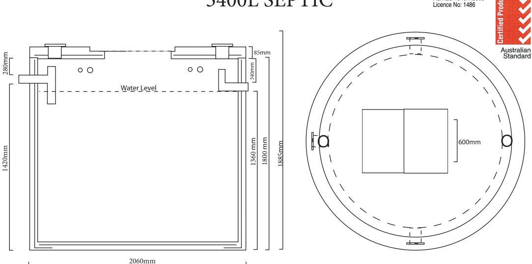
**Installation instructions:** Hole excavation must be 2.2m square with depth of 1815mm. Base must be covered with 50mm of sand or equivalent.
