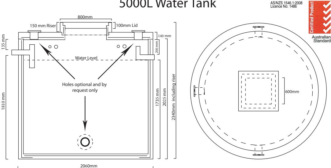
**Installation instructions:** Hole excavation must be 2.4m square. Depth to 2200mm + Riser height. Base must be covered in 50mm of sand or equivalent. Risers available in 150mm, 300mm, 450mm & 600mm. (Diagram shows tank with 150mm Riser) Inspection holes in lid and joining hole in tank are optional and manufactured only by request.
